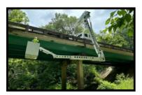
Bridge inspection requires versatility because no two bridges are exactly the same. For maximum flexibility, the Aspen A-40 New Model can be fitted with two fully-interchangeable platforms.
