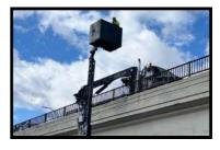
The Aspen A-40 New Model is fitted with stabilizing systems which allow operators the advantage of being able to move the truck while the platform is deployed.
