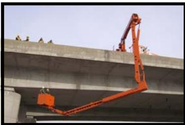
Two platform options are available. Either a telescoping boom with an articulating 4th boom and inspection platform, or a 1,500 lb 3-stage walkway can be installed.
