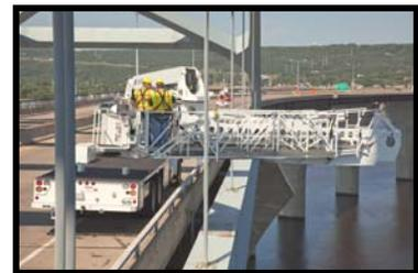
Whether you have the telescoping boom or walkway installed, the Aspen A-52 can easily maneuver around cables and steel truss members.
