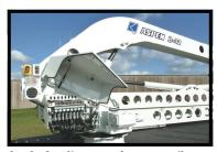
The hydraulic controls are easily assessed at the turret. The cab station includes a "Plus 1" unit interface with color monitor. Intercom stations are provided at both locations and platform.
