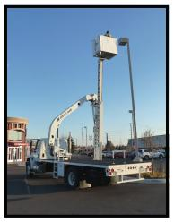
With the versatility of the Aspen B-32, overhead access is achievable whether you're operating on a bridge or not. The platform can be raised 33' above ground level. A single unit capable of being used for a variety of tasks.
