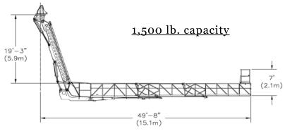
The Aspen A-52 can be equipped with an interchangeable work platform. This 43' long steel walkway can extend close to 50' horizontally under the bridge. It is kept level by means of a hydraulic leveling system and comes equipped with a "step up" platform for access behind deep girders. Wireless controls enable the workers to move the unit from anywhere along the platform.
