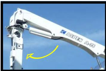
Turntable no. 2 comes equipped with an automatic leveling system, providing smooth platform movement. In addition, the operator can make manual adjustments of +/- 5 degrees to compensate for the slope of the bridge. With the elimination of the leveling arms, the Aspen A-75 has more vertical clearance to get over high fences.
